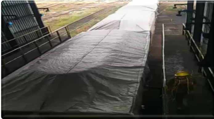
Automatic Wagon Loading System with In-Motion Wagon Tarpaulin Covering
